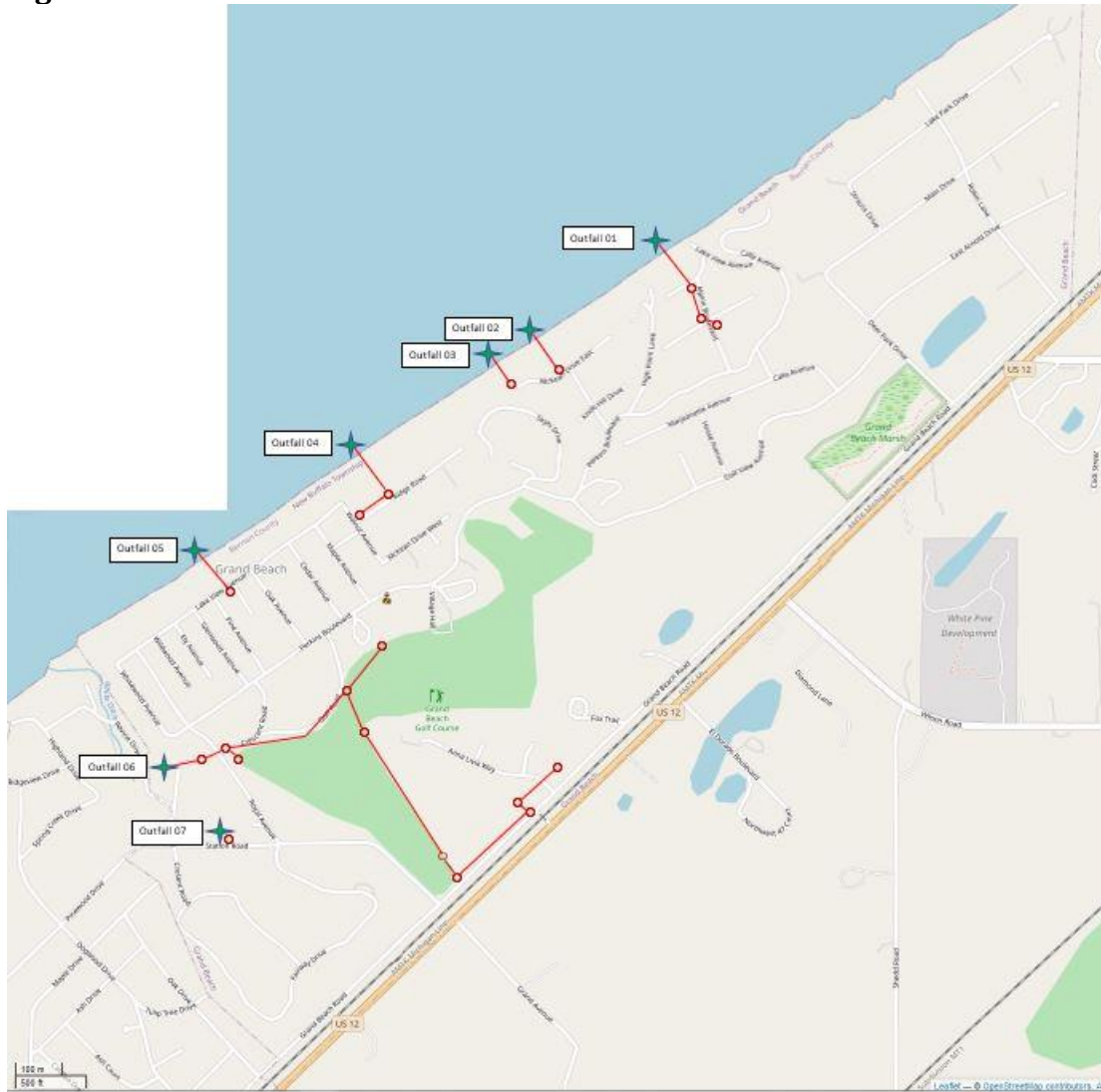
Figure 4 – Grand Beach Stormwater Outfalls and Catchbasins
